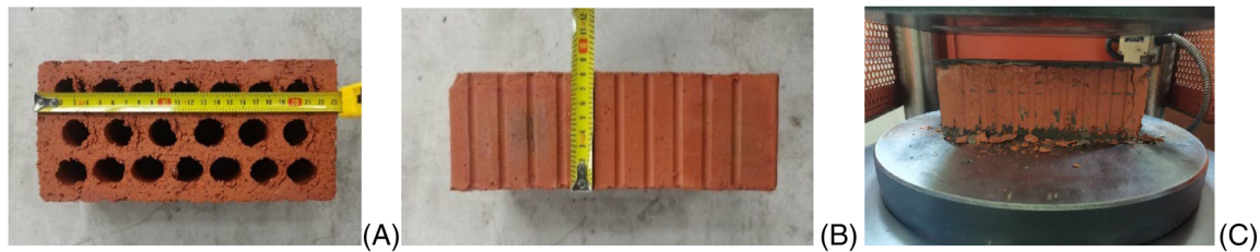
FIGURE 4 Brick units: (A) view from the top; (B) side view; (C) compressive test.
