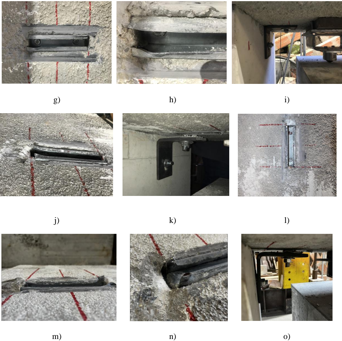
Figure 17 - Damages in the specimens from in-plane tests: a) Deformation of the angle plate CP_CT50_I_IP5; b) Failure of the channel CP_CT50_I_IP5; c) Panel after failure CP_CT50_I_IP5; d) Collapse of the anchor channel CP_CT100_I_IP6; e) Failure of the channel CP_CT100_I_IP6; f) Panel after failure CP_CT100_I_IP6; g) Channel deformation, no failure CP_CT100_S_IP7; h) Channel deformation CP_CT100_S_IP7; i) Angle plate not damaged CP_CT100_S_IP7; j) Failure of the channel CP_CT100_I_IP14; k) Collapse of the anchor channel CP_CT100_I_IP14; l) Panel after failure CP_CT100_I_IP14; m) Failure of the channel CP_CT50_I_IP16; n) Failure of the channel CP_CT50_I_IP16; o) Collapse of the anchor channel CP_CT50_I_IP16.
