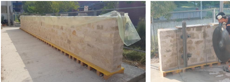
Figure 7. Finished look of the long masonry wall while curing and being cut into wallettes to be tested under diagonal compression.
