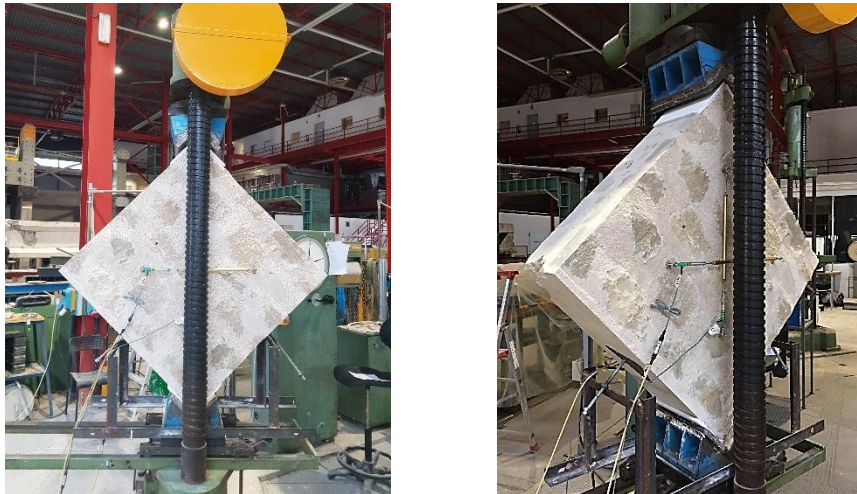
Figure 14. Diagonal compression test set-up.
