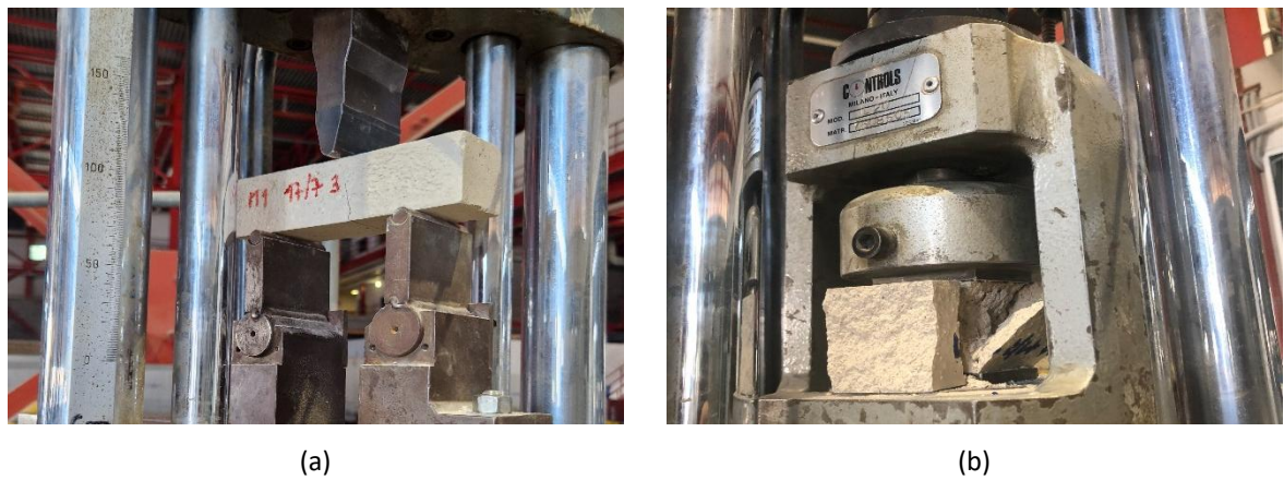
Figure 1. Mechanical characterization tests on mortar prisms: (a) three-point bending tests; (b) vertical compression tests.
