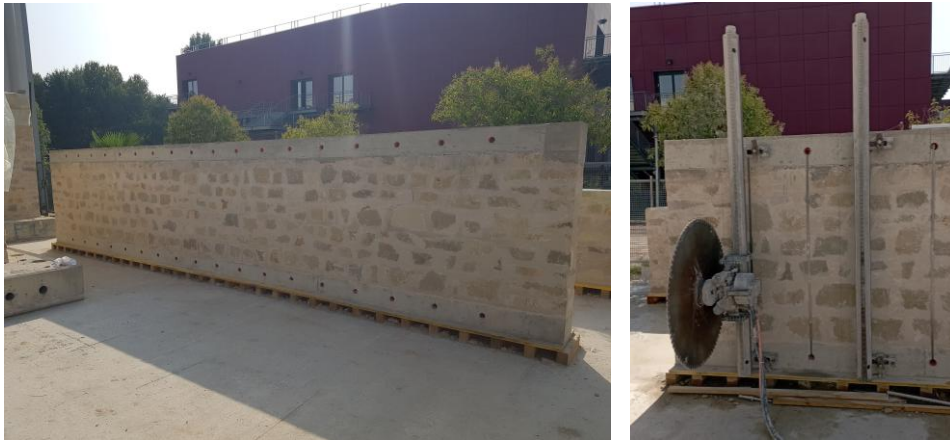
Figure 4. Finished look of the masonry long walls while curing and while being cut into wallettes to be tested under vertical compression.
