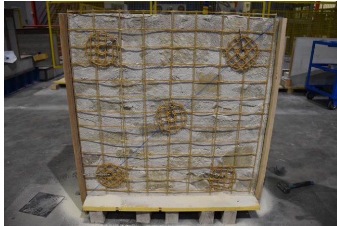
Figure 9. Jacketing system mesh and connector placement on a specimen for diagonal compression tests.
