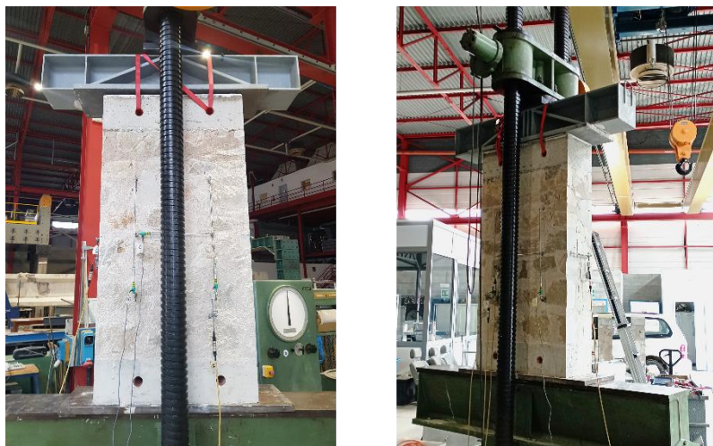
Figure 12. Vertical compression test set-up.
