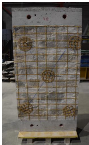
Figure 6. Jacketing system mesh and connector placement on a specimen for vertical compression tests.
