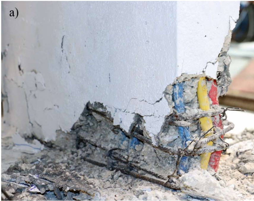
Figure 1 Failure locations of unit UWS2 at the base of Flange Two after GM8. The longitudinal rebars were wrapped in colored heat shrink plastic for the purpose of electrical insulation with the rebar cage, and to promote debonding.
